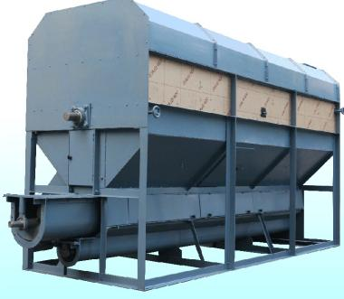
This machine fabricated from heavy duty steel frame, drum having perforation lining with spiral blade for material movement & separation.
